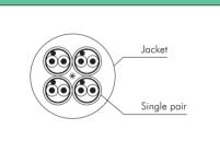
• Each pair consists of two insulated twisted conductors and drain wire enclosed within a high-density spiral copper shield.
