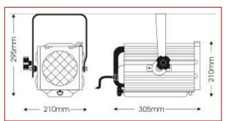
Quality 500/650W PC spotlight ideal for professional usage in smaller venues. The well-defined beam is adjustable by a screwfocus mechanism, and the design also includes a hinged lamp-tray and a double-microswitch interlock for safe lamp replacement.
