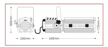
Compact and high-specification 500W/650W profile spotlight with a double-condenser zoom focus optical system to provide crisp projection of gobos and a brilliant flat beam between  $10^{\circ}$  and  $28^{\circ}$ .
