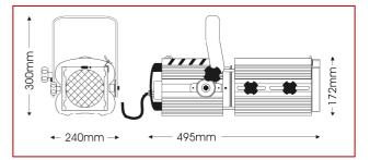
This versatile 500W/650W profile spotlight, designed for shorter throws, has a double condenser zoom focus optical system to provide crisp projection of gobos and a brilliant flat beam of between 20° and 40°.
